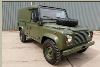
Land Rover Titonus 110 Defender Hard Top , Fitted 2.5ltr NAD engine, 5 speed gear forward and one reverse gear box, Hi/Low transfer box, Centre Diff lock, Front disc brakes, Rear drum brakes, etc. Mileage from 22,000 kms. Excellent condition. Guide Price for RHD £5,000 to £7,500, Guide Price for LHD £6,500 to £8,500 (20 Available)
