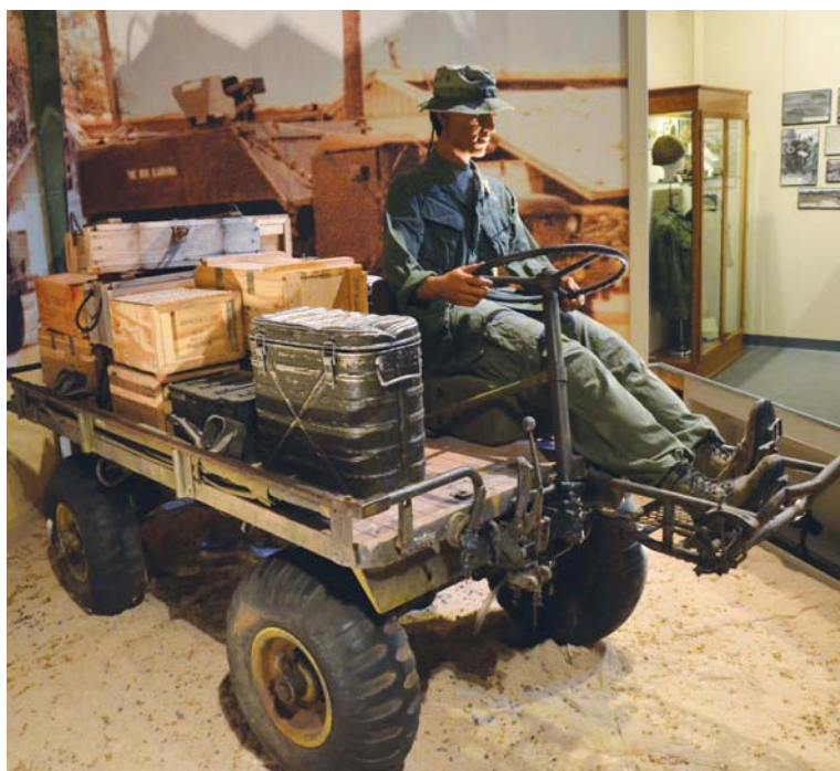
Far right: the M274 Mechanical Mule's versatility was amazing. It could be used for signal cable reel carrying, as a boat for river crossing, fitted with a recoilless rifle, and even fitted with TOW missiles.
