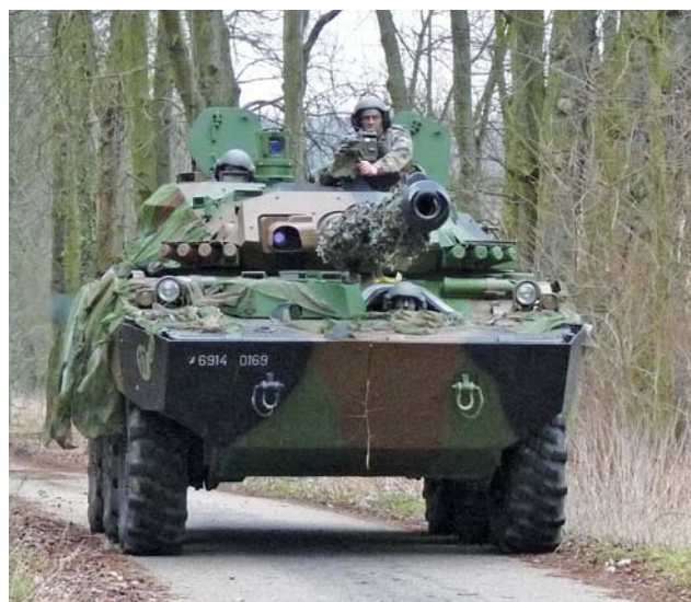
Above: head-on view of an AMX-10RC seen here moving along a track during an exercise. The AMX-10RC has an endurance of 800 kilometres or 17 hours. Note that the vehicle has been draped in camouflage netting.
