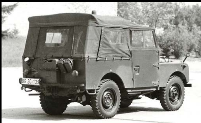
Above: on the 86-inch models the spare wheel was moved to the bonnet.
