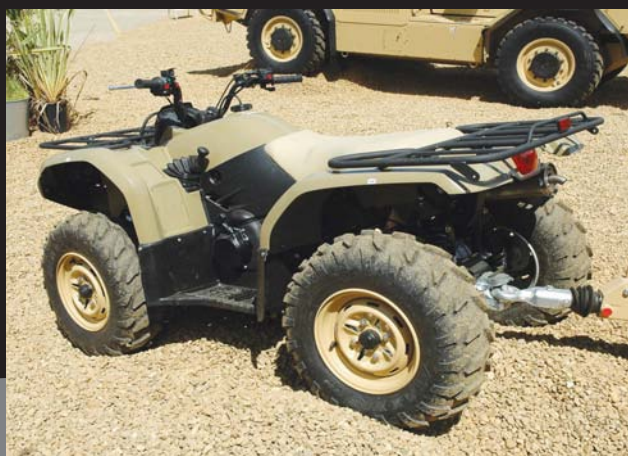
Above: the wheels on the Yamaha are different widths with different size tyres, which can be deceiving if buying replacement wheels and tyres. This is an early production military spec Yamaha quad displayed at DVD in 2008 and is missing some of military-specific fittings.
