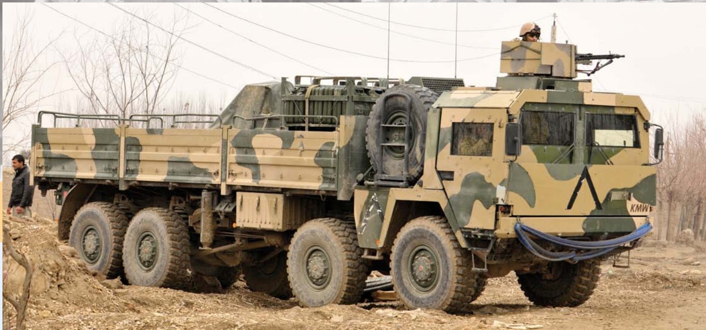
Above: in Afghanistan, a Kat 1 10-tonne cargo with winch, materials handling crane and first-generation KMW cab protection.
