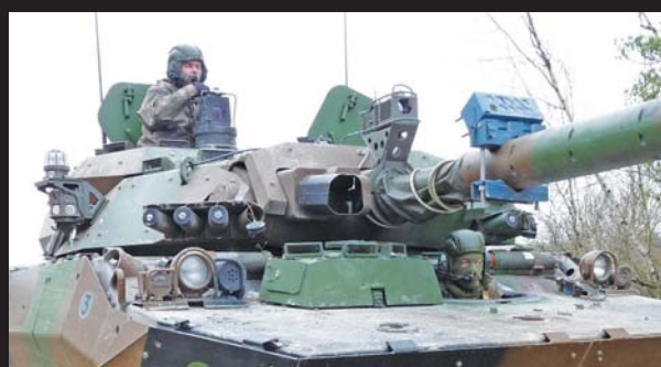
Above: close-up of the turret. Note the simulation systems in blue and grey on the gun and each side of the turret.
