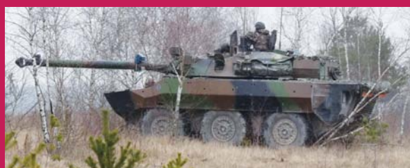
Top right: AMX-10RC of the 3e Régiment de Hussards photographed at Djibouti in 2010. Note that the vehicle has not been modernised like those serving in France, as evidenced by lack of the extra turret bustle at the rear of turret, which saw the smoke grenade launchers moved to the front. (Photo courtesy - 3e Régiment de Hussards)
